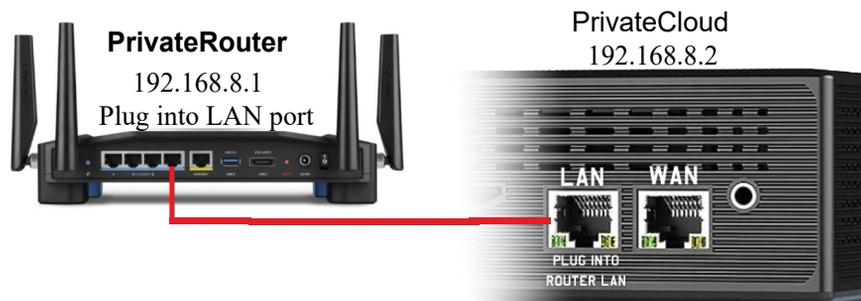
After enabling Side Router mode and connecting the LAN ports of both devices, you can now access your PrivateCloud device at the IP address 192.168.8.2 when you're connected to the main PrivateRouter WiFi network.
